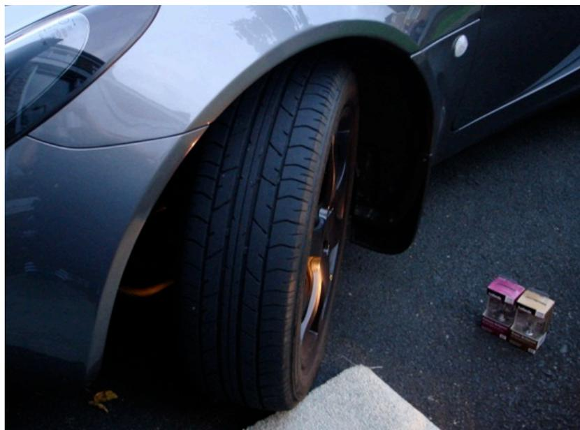
2. Initially I removed the lower part of the wheel arch liner as I was unsure exactly which screws needed removing. As it turned out these three screws are all you need to remove.
