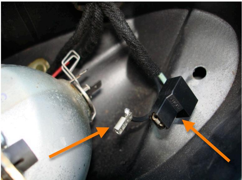
6. Unhook the two silver clips holding the bulb in place.
